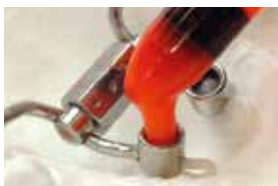
Squeeze composite into the collar
